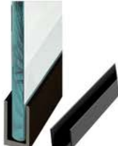
DFGL-UPR-11 BM 'U' Channel Size : 25x13x25 and 25x13x35mm Ythickness 1.6mm Length : 3.4mtr (11.25ft)
